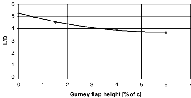
Fig. 5 Effect of Gurney flap height on lift-to-drag, \alpha = 15^\circ .
